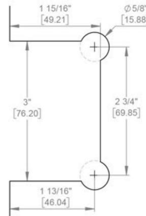
Cutouts provide 1/16-1/4" clearance between glass and wall
